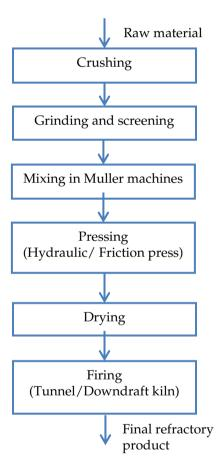
Process flow chart for refractory manufacturing
