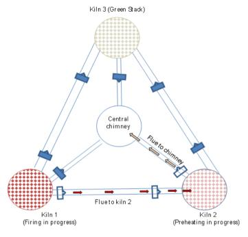
Figure: Schematic layout of integrated DD kilns with central chimney
